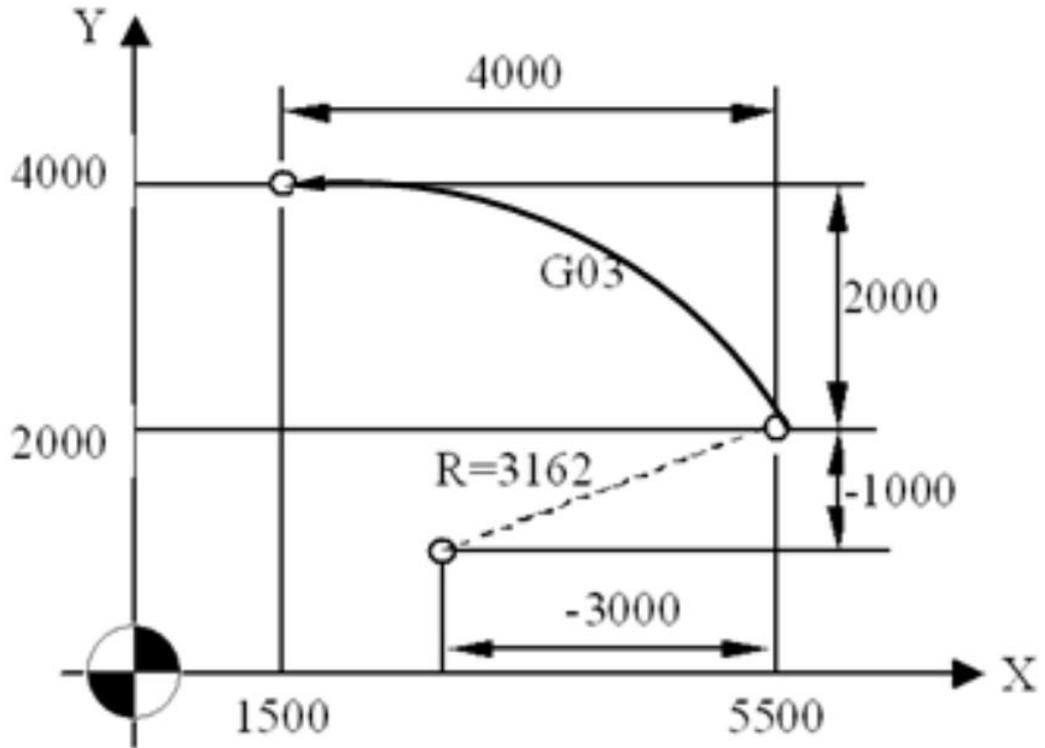
**Figure 50: Circular interpolation example 1**
