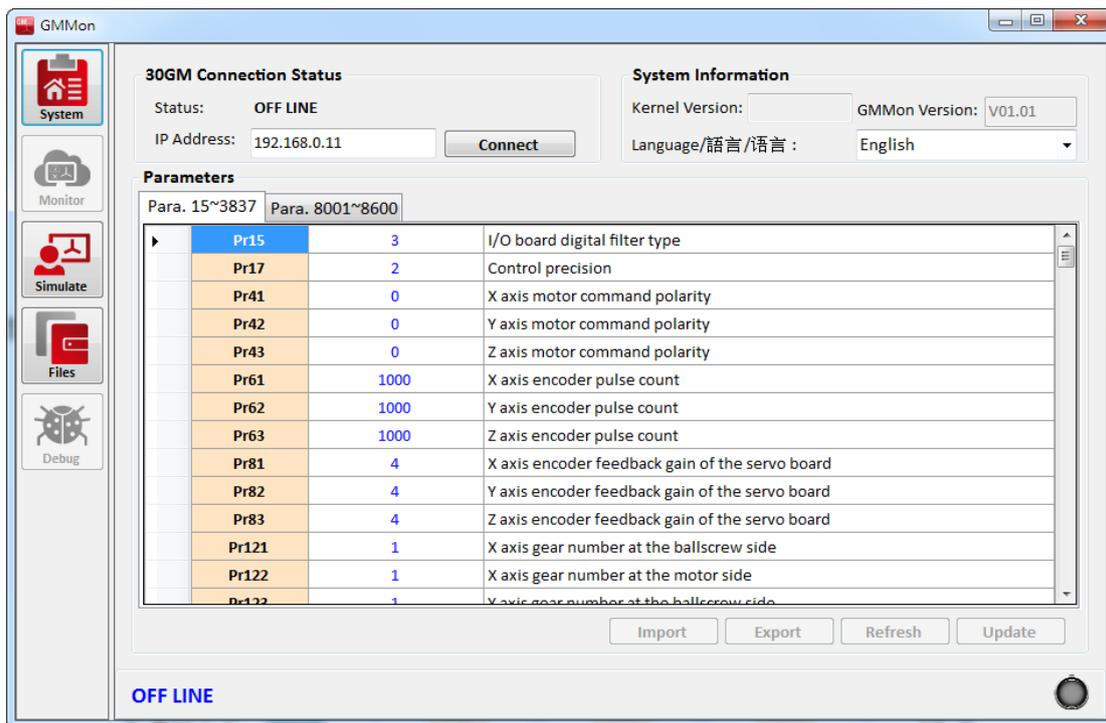
**Figure 33: Use GMMon to set up operating parameters**
