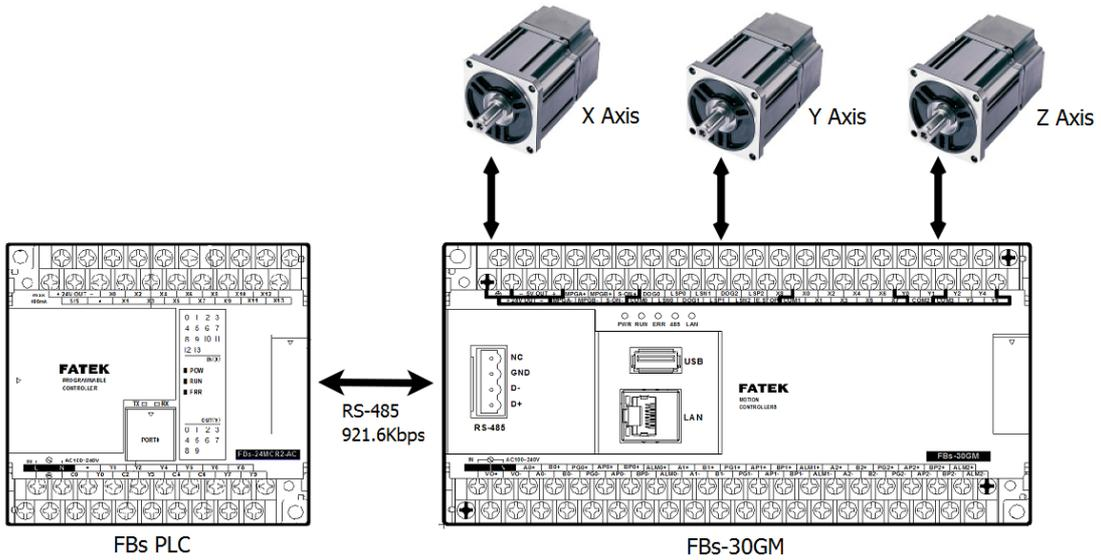
**Figure 30: Relation between FBs PLC and FBs-30GM**
