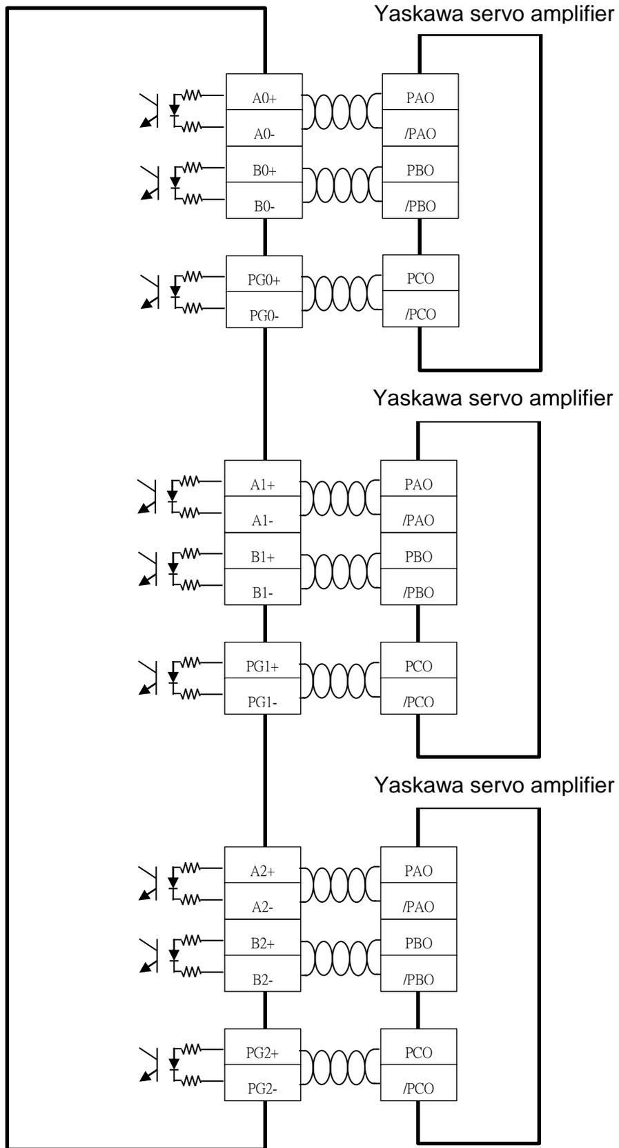
**Figure 10: Connecting feedback signals from Yaskawa servo amplifier**
