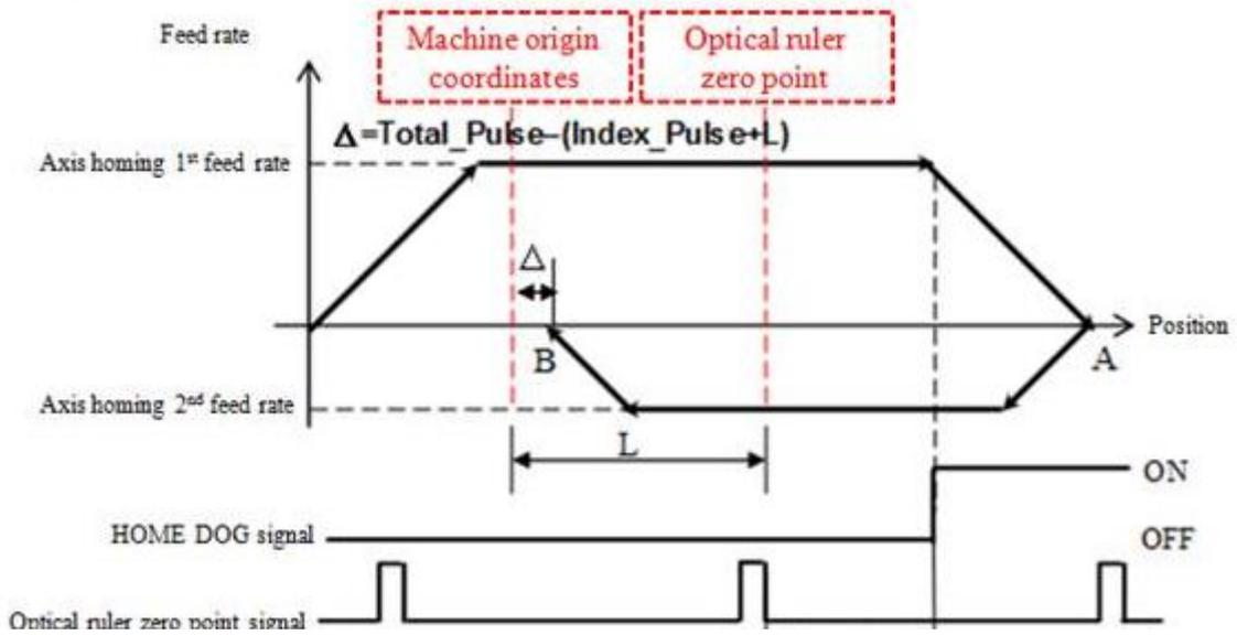
Figure 42: V-X diagram of dual feedback, Pr961=0 or 1 and Pr881=L
