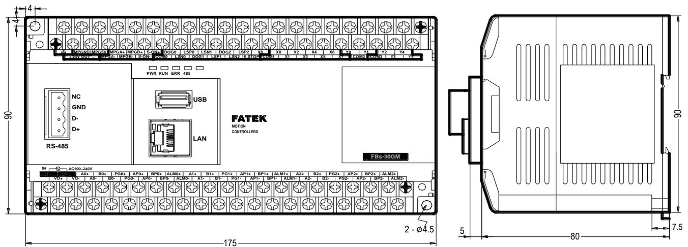
Figure 1: The dimensions of FBs-30GM
