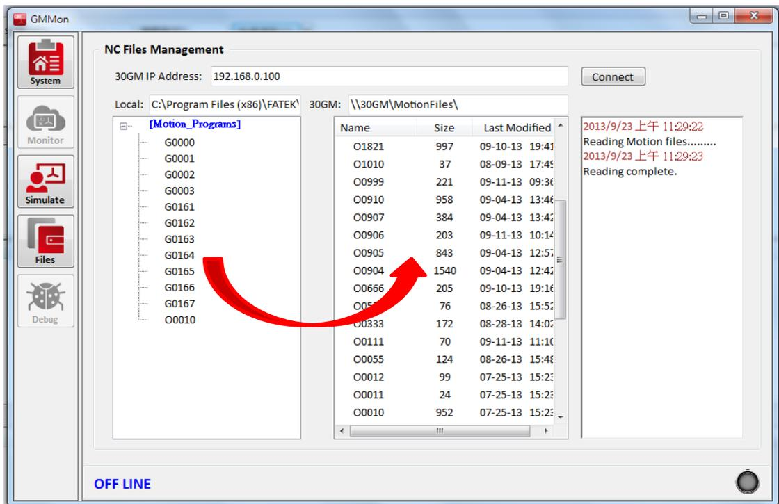
Figure 32: Drag and drop the file to upload
