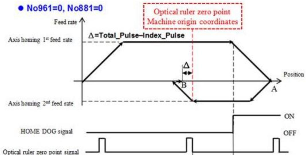
**Figure 41: V-X diagram of dual feedback, Pr961=0 and Pr881=0**
