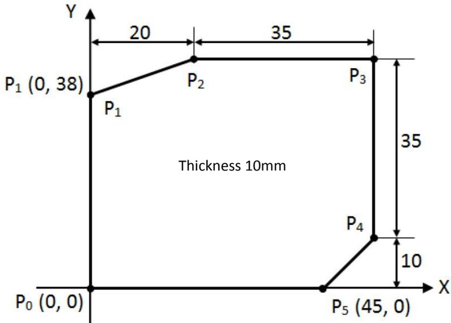
**Figure 46: G01 linear interpolation example 2**
