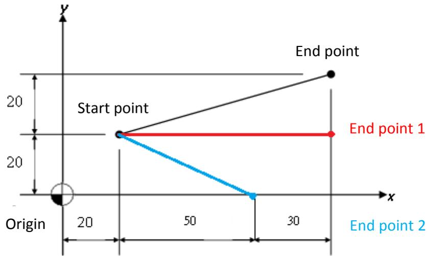
**Figure 62: G161 linear interpolation compensation example**
