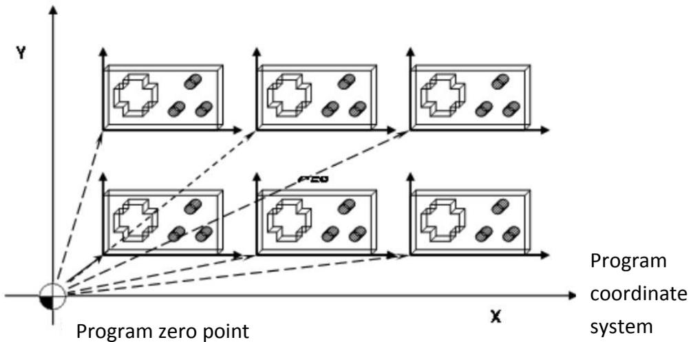
**Figure 59: Program coordinate system setting example**
