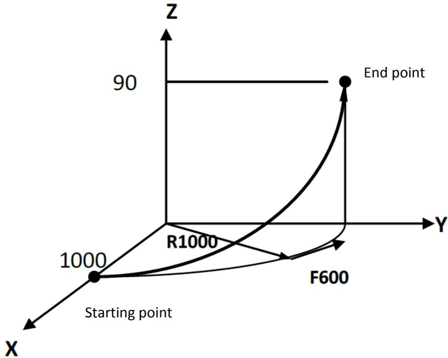
**Figure 52: Helical interpolation**
