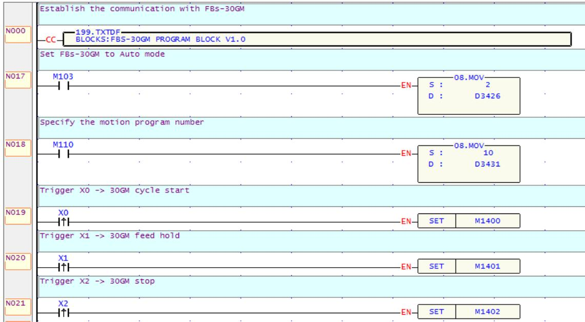
**Figure 35: Example of Auto mode ladder diagram**
