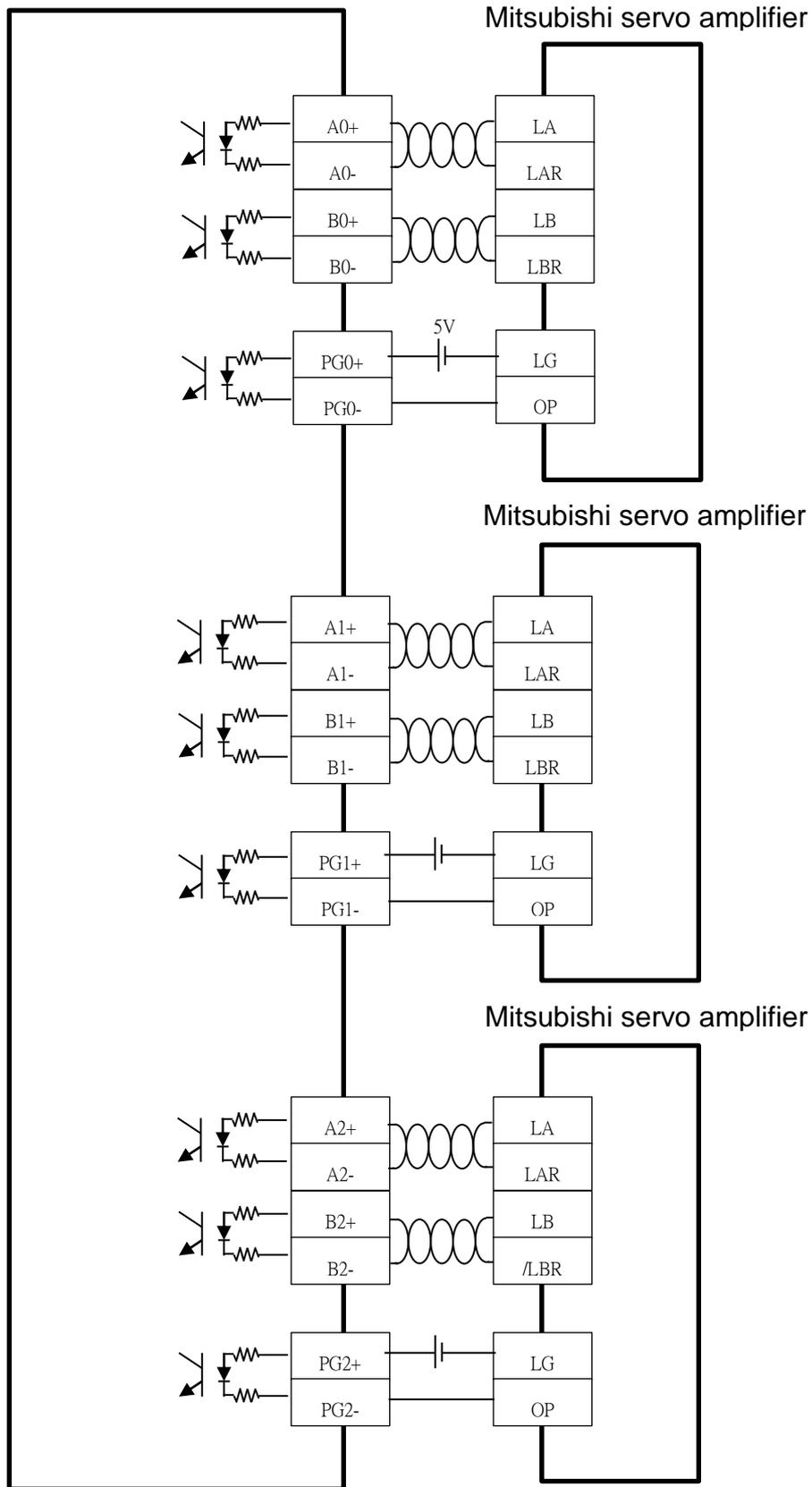
Figure 12: Connecting feedback signals from Mitsubishi servo amplifier
