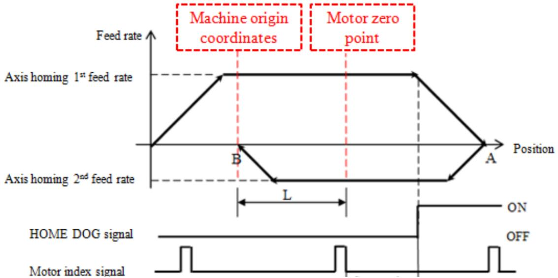
Figure 39: V-X diagram of using motor feedback, Pr961=0 or 1 and Pr881=L
