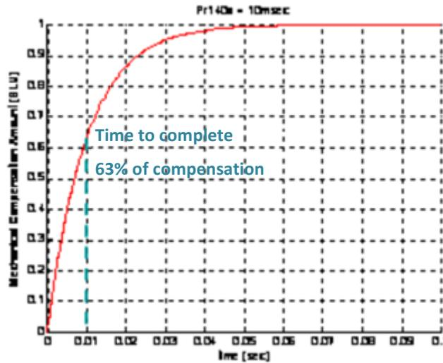
Figure 73: Mechanical compensation amount vs time
