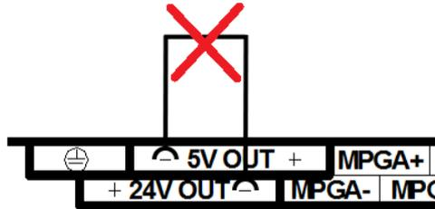
Figure 7: Improper wiring
