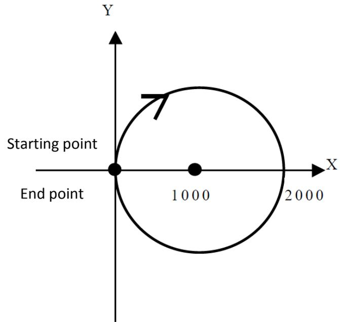
**Figure 51: Circular interpolation example 2**
