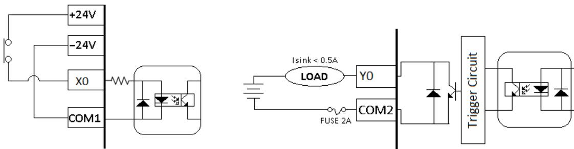
**Figure 4: Input and output points wiring**
