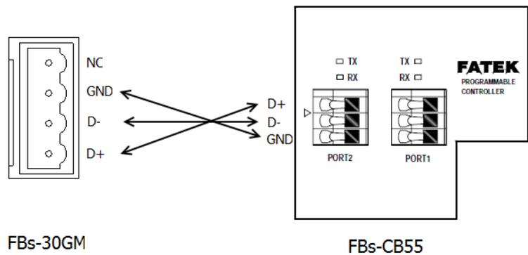
Figure 6: Connection between FBs PLC and FBs-30GM (with CB55)
