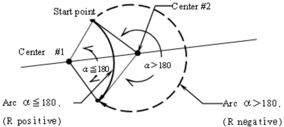
Figure 49: Circular interpolation of different  $\theta$
