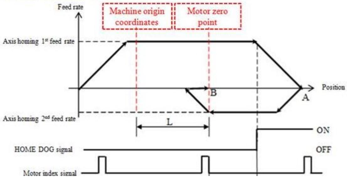
Figure 40: V-X diagram of using motor feedback, Pr961=2 and Pr881=L
