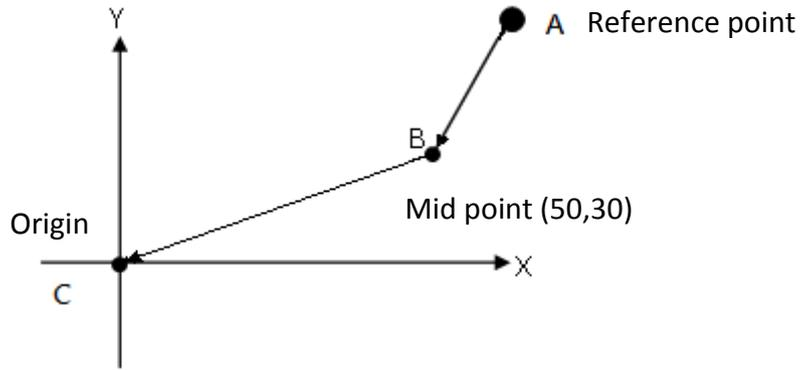
**Figure 56: G28 return to reference position example1**
