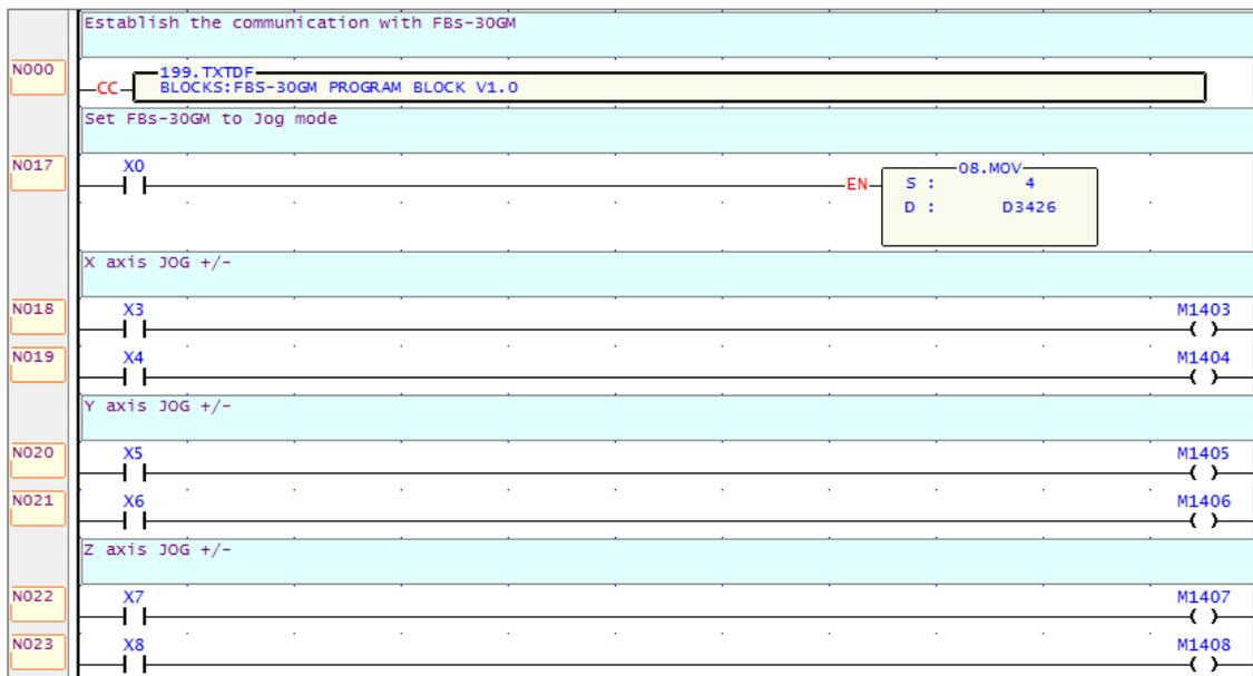
**Figure 34: Example of JOG mode ladder diagram**
