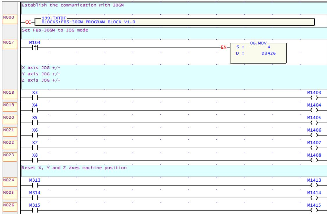
Figure 36: Example of FBs PLC ladder diagram
