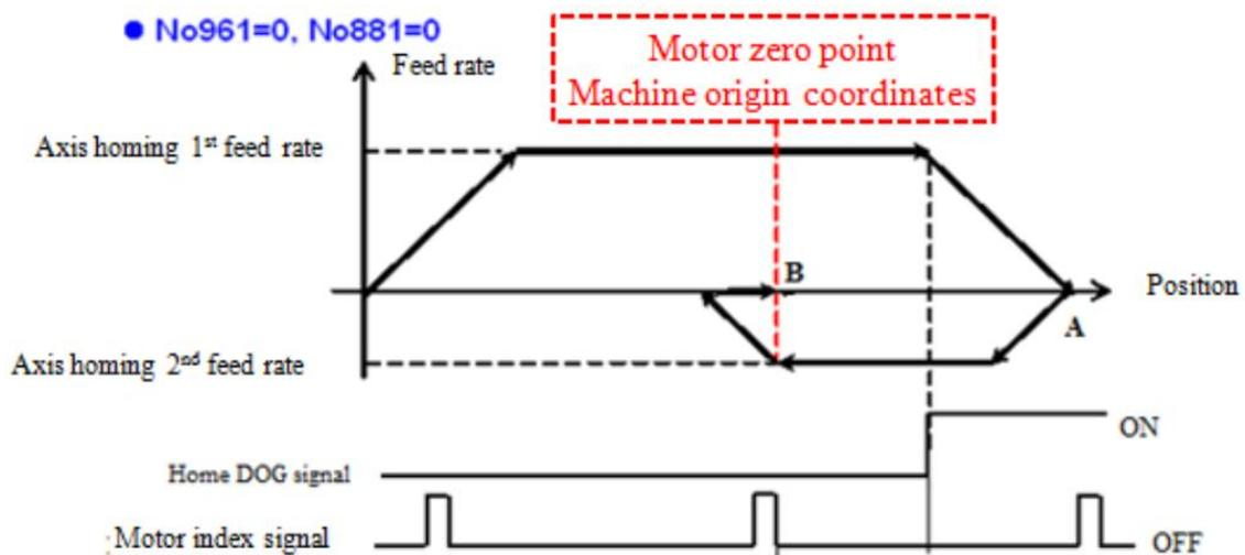
**Figure 38: V-X diagram of using motor feedback, Pr961=0 and Pr881=0**
