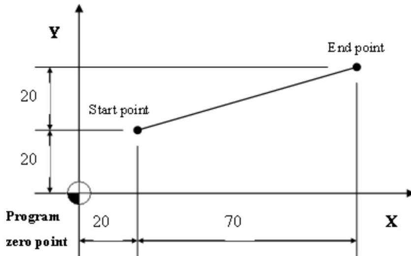
**Figure 45: G01 linear interpolation example 1**
