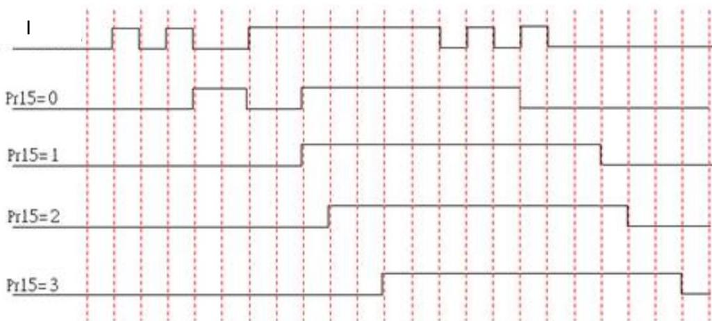
Figure 67: I/O board digital filter
