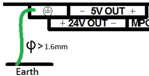
Figure 8: Selecting the grounding wire
