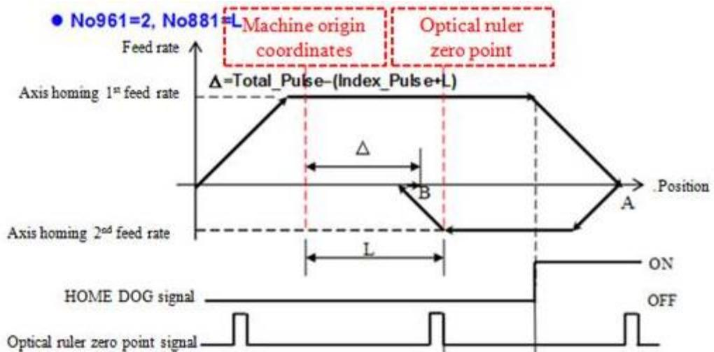
Figure 43: V-X diagram of dual feedback, Pr961=2 and Pr881=L
