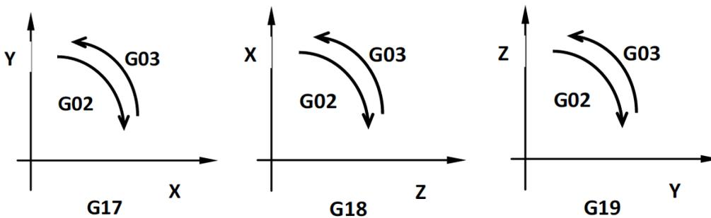
**Figure 54: G17, G18, G19 setting interpolation plane**
