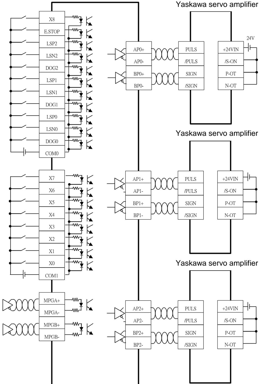
Figure 9: Wiring example with Yaskawa servo amplifier
