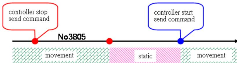
Figure 74: Static dual feedback error timeout
