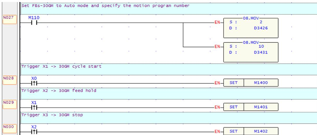
Figure 37: Example of FBs PLC ladder diagram (cont.)
